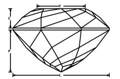
**SPINWHEEL** Ed. Hume 6/67 Angles for R.I. = 1.720 73 + 8 girdles = 81 facets 8-fold radial symmetry 96 index L/W = 1.000 T/W = 0.497 U/W = 0.497 P/W = 0.439 C/W = 0.205 Vol. /W<sup>3</sup> = 0.274
